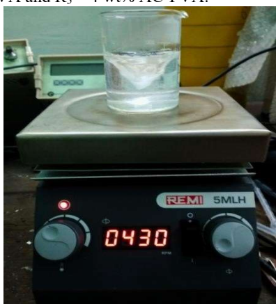
Fig. 2. PVA solution under continuous stirring at the rate of 430 rpm
