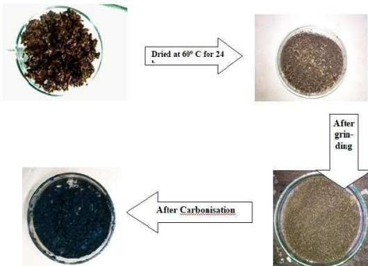
Fig. 1. Flowchart of digital images of synthesis of KOH activated carbon
